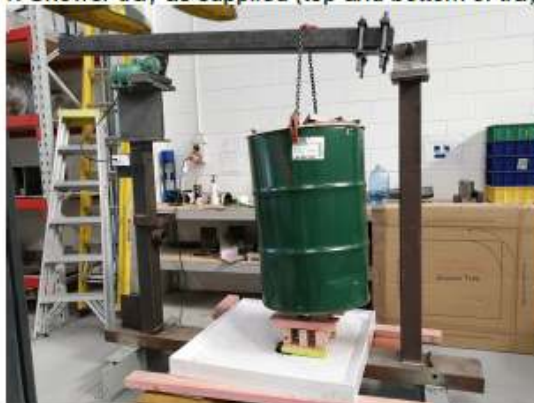
Figure 2: Testing conducted on cyclic loading frame
