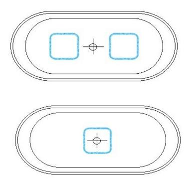
In some installations you may find that best position for the floor waste is in center under the bath waste position, (as image below) This enables you, once a floor waste is fitted and with the addition of a dropper from the bath waste to just lower the bath into position.
