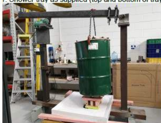
Figure 2: Testing conducted on cyclic loading frame
